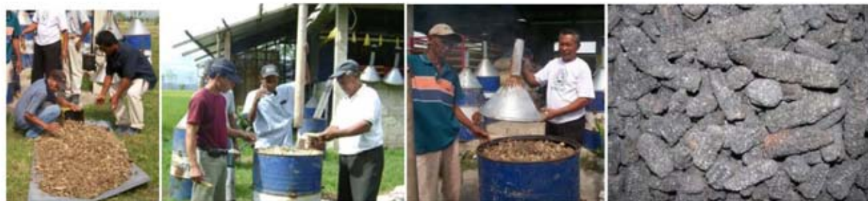
Drying of corncobs and carbonization using a drum kiln
