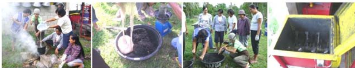
Mix the ground corncobs with the binder.
