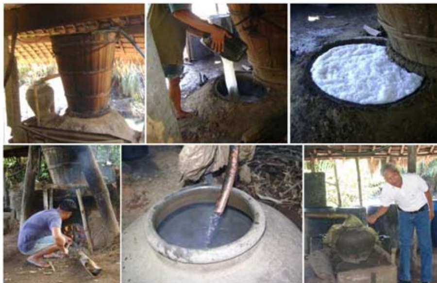
The distillation process
